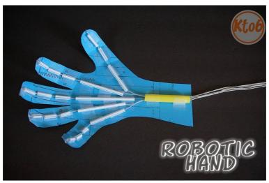
Figure 7: An example of a robotic hand with straws and strings attached to each finger.
