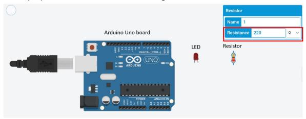
6. We will now connect the circuit as shown below. We will connect the negative leg (or the shorter, straight leg) of the LED to one side of the resistor.
