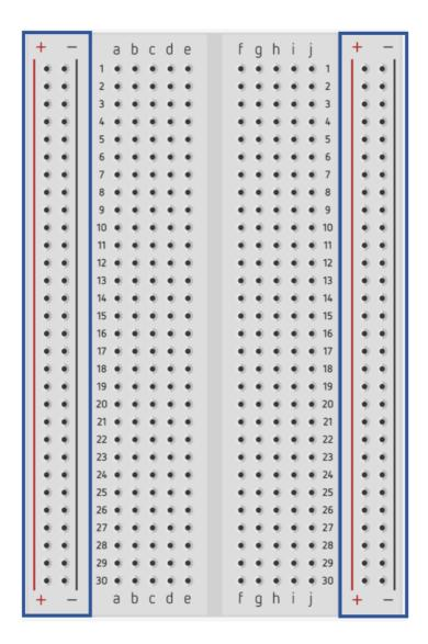
Hover your mouse over a row in the middle of the breadboard, you will see the entire row is highlighted in green. This means that they are electrically connected to one another.
