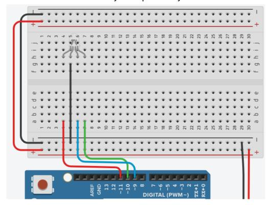
• If you remove any resistor, then click "Start Simulation", you may notice some very interesting patterns. For example, if you remove the resistor that is connected to the "Red" LED, you probably cannot see an output colour of red, or any colours that have the primary colour as red. Can you explain why this is the case?
